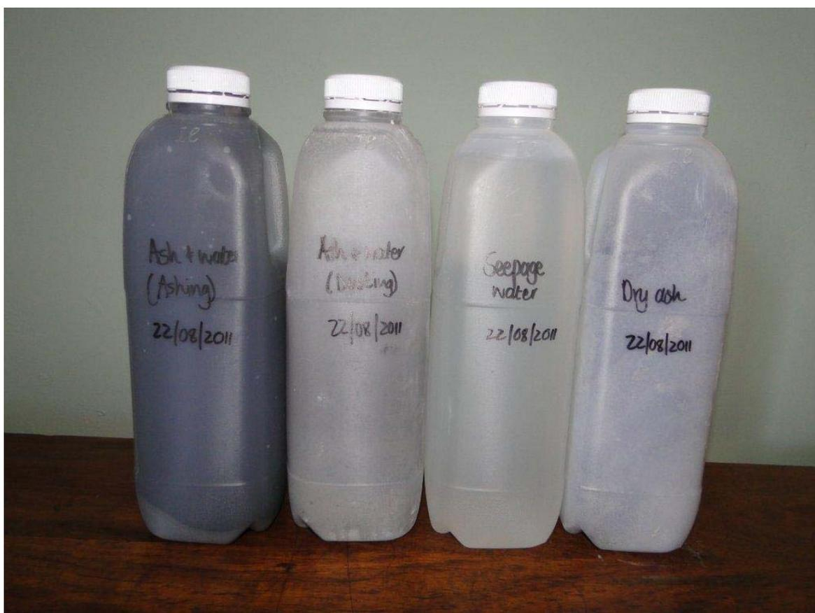
**Photo 1:** Four samples used in the assessment of the Camden Power Station Ash, Ash Carrier Water and Ash Disposal Facility Seepage Water (Leachate)
